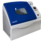
CORROSION TESTING SALT SPRAY TEST ( Make ASCOTT , UK)
